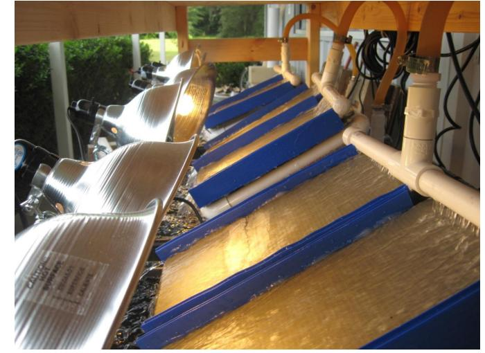
Figure 3: Side View of Experimental Photo-Bioreactor Setup
